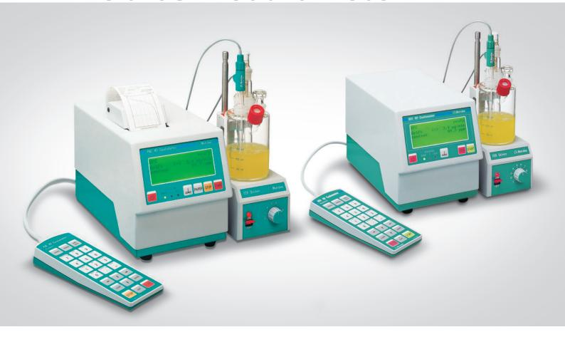
Water determination down to trace levels
