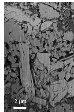
\text{LiMn}_2\text{O}_4 cathode material of a lithium ion battery. Close-up of cross-section shows surface information on an Inlens SE image and unique, pure materials contrast with an Inlens EsB image. The distribution of lanthanum (red) and manganese (green) is derived from an EDS map (from left to right).
