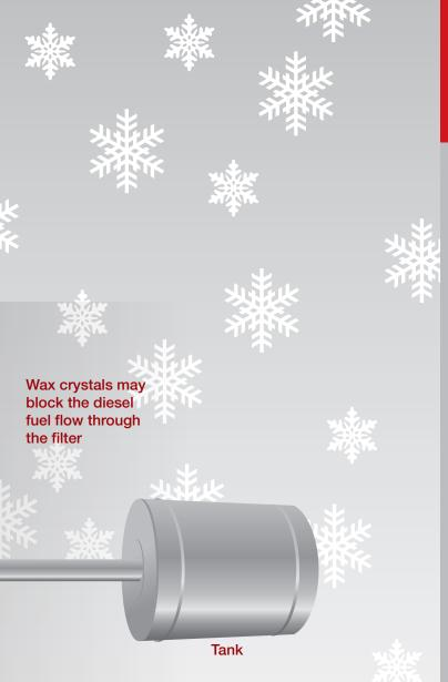
These wax crystals may plug the fuel filter, making it impossible for the fuel system to deliver fuel to the engine.
