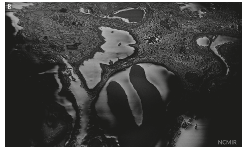
Block-face images of mouse lung tissue (A) with Focal Charge Compensation and (B) without Focal Charge Compensation. Scale bar: 1 micron. Images: courtesy of NCMIR.
