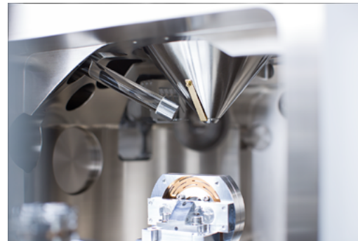
GeminiSEM 500 offers a nano-twin lens for improved resolution at low beam voltages.
