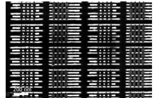
FinFET transistor, top view, 22 nm technology, 3 kV, pure BSE imaging using EsB, high material contrast.
