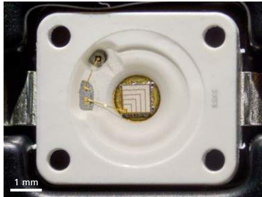
High brightness LED, chip, bond wires and packaging, Spot K LED, oblique reflected light, zoom 1.25x
