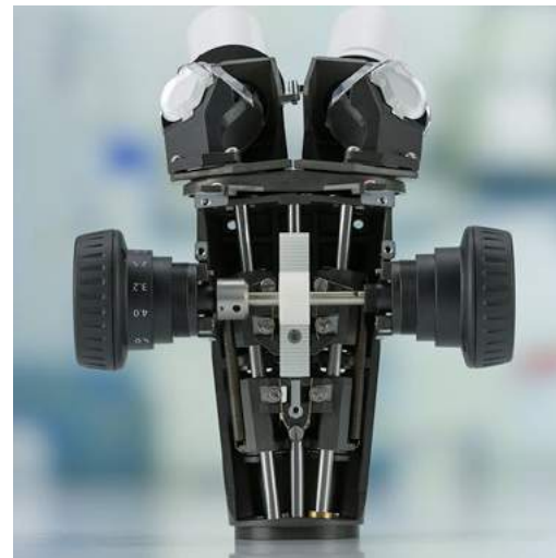
Stemi 508 is a Greenough type stereo microscope with twin body tubes, inclined by 11^\circ – featuring a powerful 8:1 zoom
