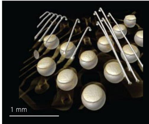
Large flip chip (10x10x1 mm) imaged at high resolution
