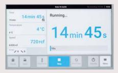
Program function: Quickly access frequently-used protocols for increased efficiency and repeatable results
