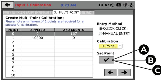
Figure 10: One-Point Calibration
